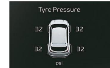
Displays real-time tyre pressure information and alerts if the pressure falls below the recommended levels
