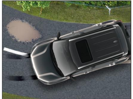
Prevents wheel lock-up and skidding to improve vehicle control by sensing and compensating for over braking
