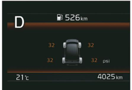
Continuously monitors air pressure in each tyre and alerts you in case of a drop below recommended levels
