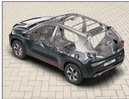
Offers enhanced safety as more than 2/3<sup>rd</sup> of structure is made from high strength steel
