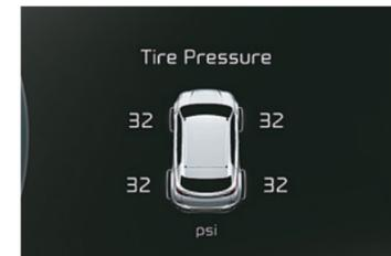
Displays real-time tyre pressure information and alerts if the pressure falls below the recommended levels
